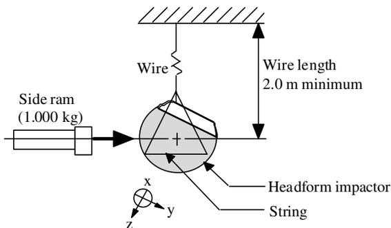
Figure 11. Setup for headform impactor high-velocity certification test.
