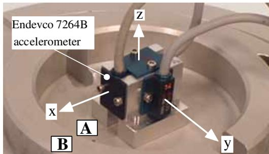
Figure 3. Accelerometers mounted on JAMA-JARI headform impactor.
